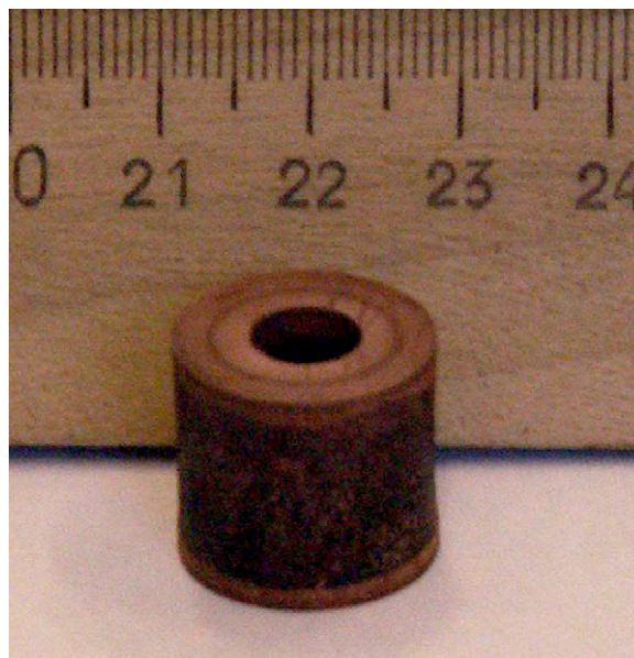
Fig. 3. Hollow cylinder of permeable composite material based on the NM-1 catalyst.
